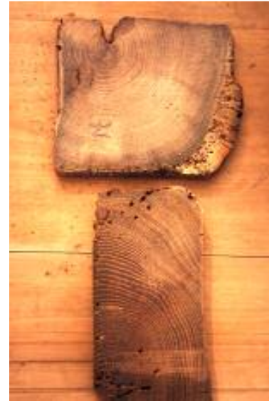
Cross-section of oak showing the attack of common furniture beetle concentrated in sapwood
